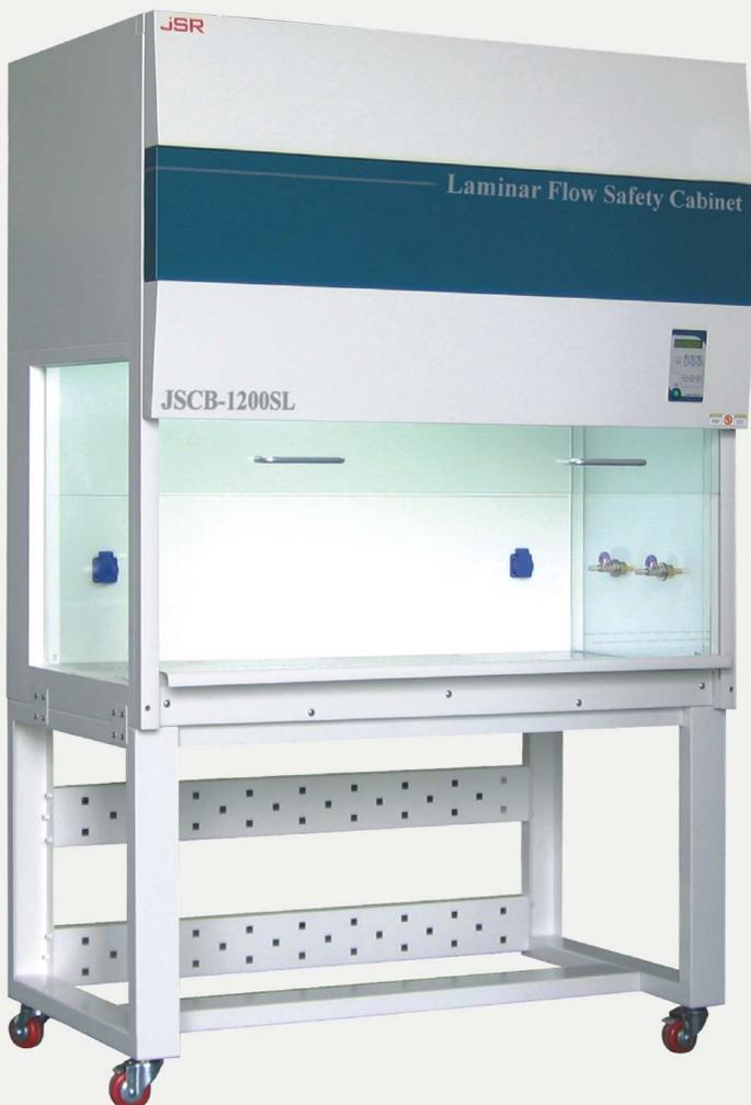
Vertical Laminar Flow Cabinet enclosure designed to maintain ISO Class 5 (formerly Class 100) clean air. HEPA filtered laminar air down flow over the work area to protect products or samples being handled in the cabinet from dust or biological contaminants such as bacteria, fungus and genetic materials.
